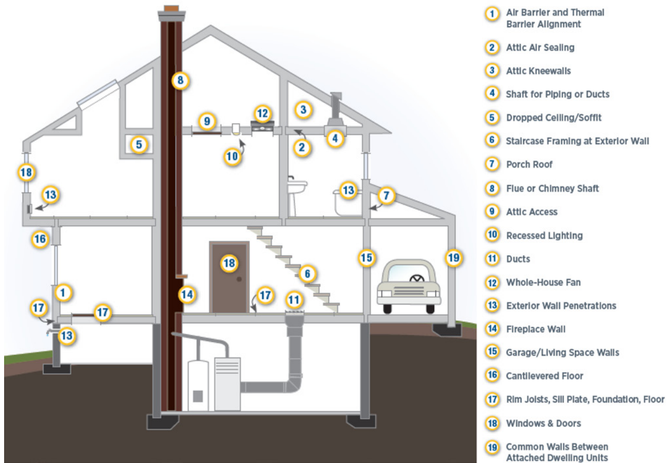
Figure 4: Building America—air sealing trouble spots
