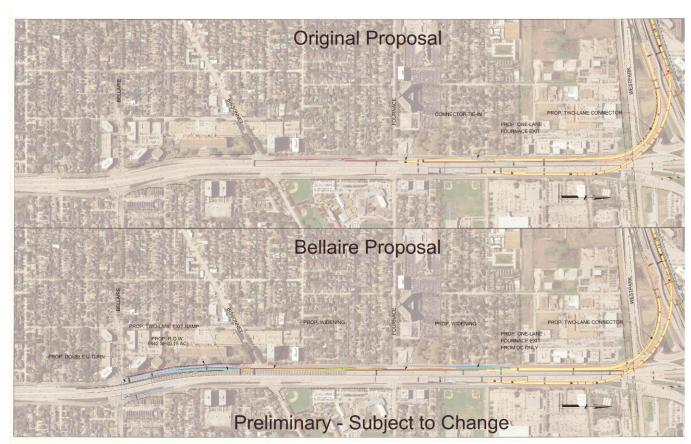
The Bellaire Proposal still includes a two lane direct connector from US59 northbound to IH610 southbound, but without the elevated section. It will approximately follow the vertical alignment of the existing direct connector and allow for vehicles traveling US59 north bound to IH610 southbound to exit Fournace as they do today.
