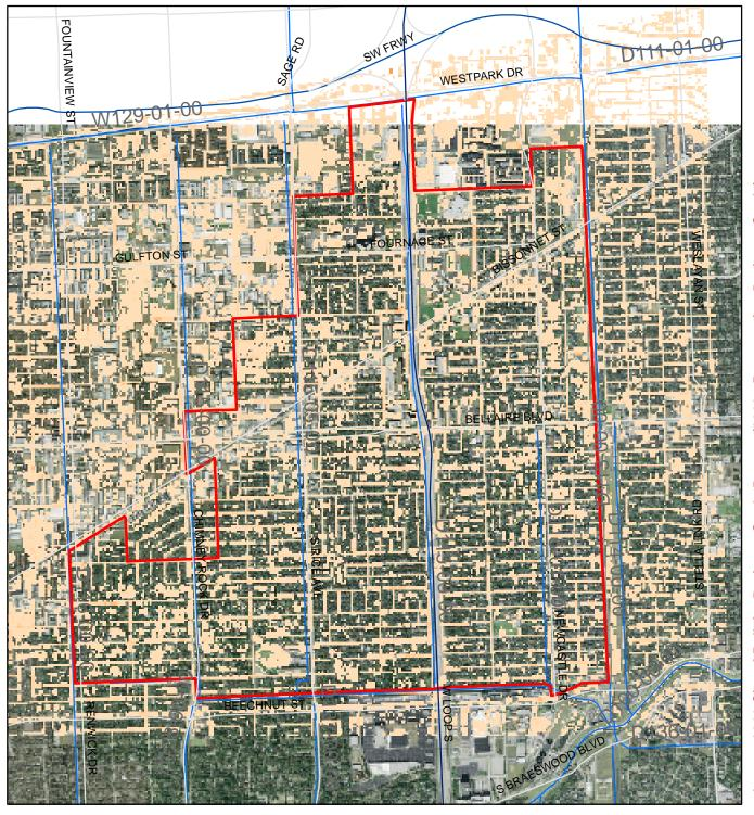
Results of flooding above 0.5-foot from 2-D Model for 2-in/hr Rainfall-Low areas with water
