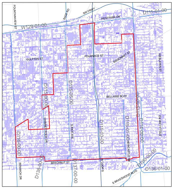
Results of flooding from 2-D Model for 4-in/hr Rainfall-Low areas with water
