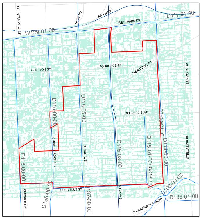
Results of flooding from 2-D Model for 3-in/hr Rainfall-Low areas with water
