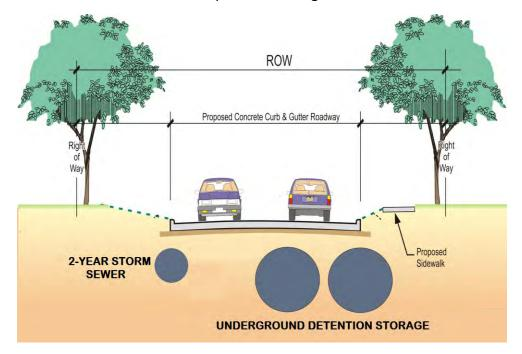
Figure 5- Underground Detention
