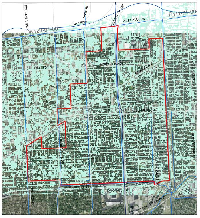
Results of flooding above 0.5-foot from 2-D Model for 3-in/hr Rainfall-Low areas with water
