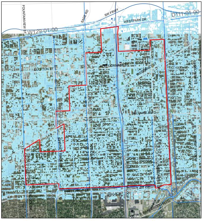
Results of flooding above 0.5-foot from 2-D Model for 6-in/hr Rainfall-Low areas with water
