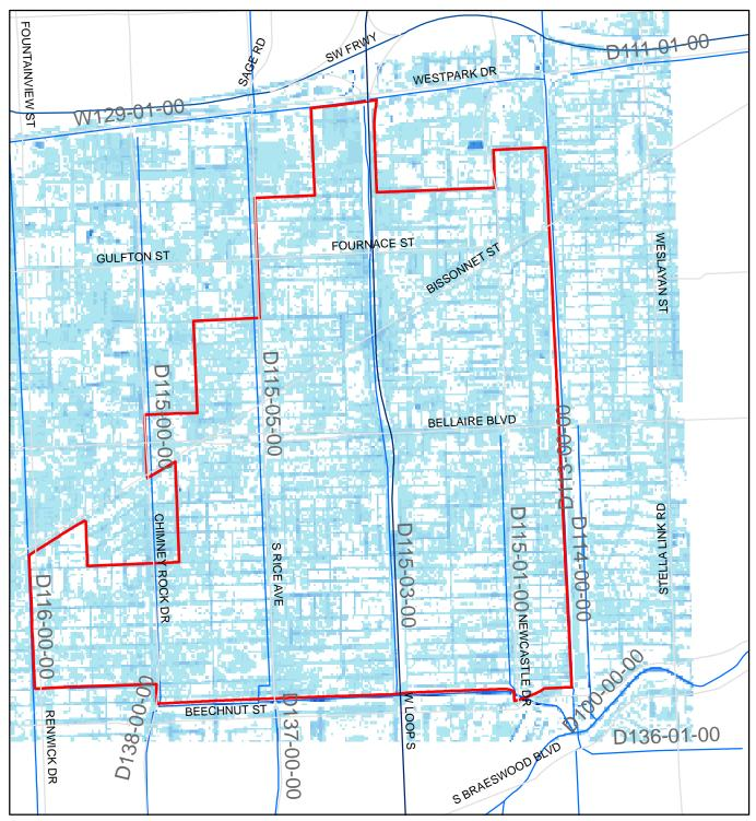
Results of flooding from 2-D Model for 6-in/hr Rainfall-Low areas with water
