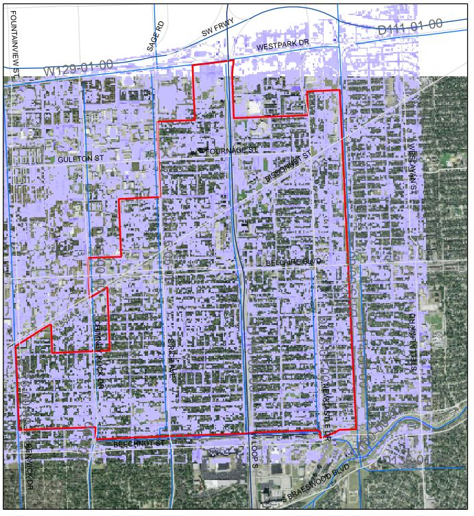
Results of flooding above 0.5-foot from 2-D Model for 4-in/hr Rainfall-Low areas with water
