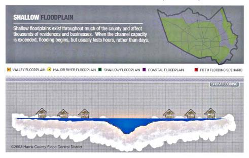
Figure 2- HCFCD Shallow Floodplain (Source HCFCD)
