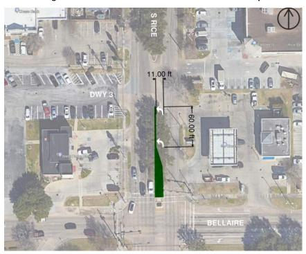
Image 2: NB Left Turn Lane Schematic at S Rice and Driveway 3
